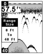
Range Size menu with manual depth range set to 40 feet. This in effect "zooms" or enlarges the display to show the water column from 0 to 40 feet deep. In this figure, the boat is in 57.5 feet of water, but only the top 40 feet of the water column is shown on the screen.
